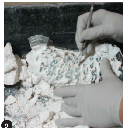
9 After the mold has cooled, material is carefully removed to reveal the finished piece.
