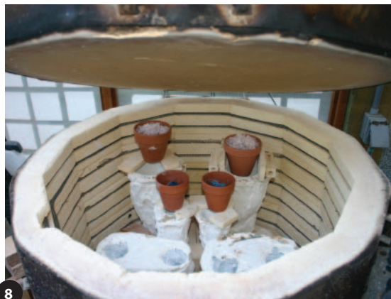
8 The mold is placed in a kiln upside down and lead crystal "frit" or chunks are placed in the mold or in a flowerpot above the mold. The kiln temperature of 1,530°F melts the glass into the mold.
